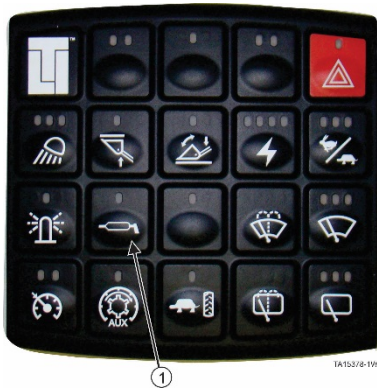
1) Lubrication Cycle Switch on overhead panel in operator cab
