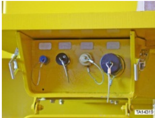
Figure 3. Central service system (optional) - typical
